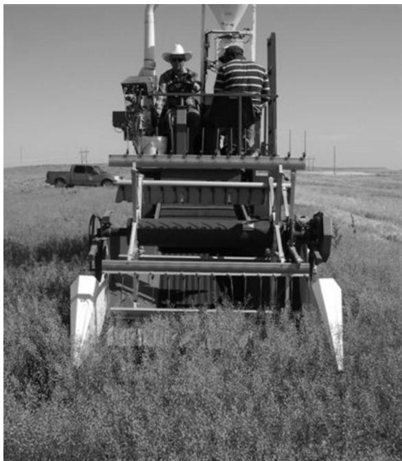
**Figure 2.** Harvesting camelina with a small-plot combine at SAREC.
